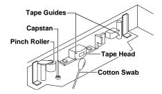
5. When you finish cleaning, press **STOP** and close the compartment door. Then reconnect power.
